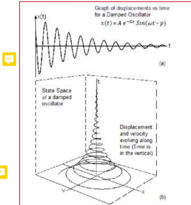
**Figure 1:** (a): gradual time development  $x(t)$  of any oscillation for a sub-critically damped oscillation, (b): the corresponding State Space, this is the 3D-plotting of displacement and velocity versus time. Notice that the distance between turns in the state space orbit is constant, which means that the oscillations are uniform. In chaotic oscillations these turns are messy and unpredictable.
